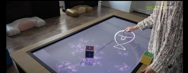
When you put down a cube, the user's drawing moves and the color of the moving picture changes whenever the side of the cube changes. (Two cubes can be used simultaneously)
