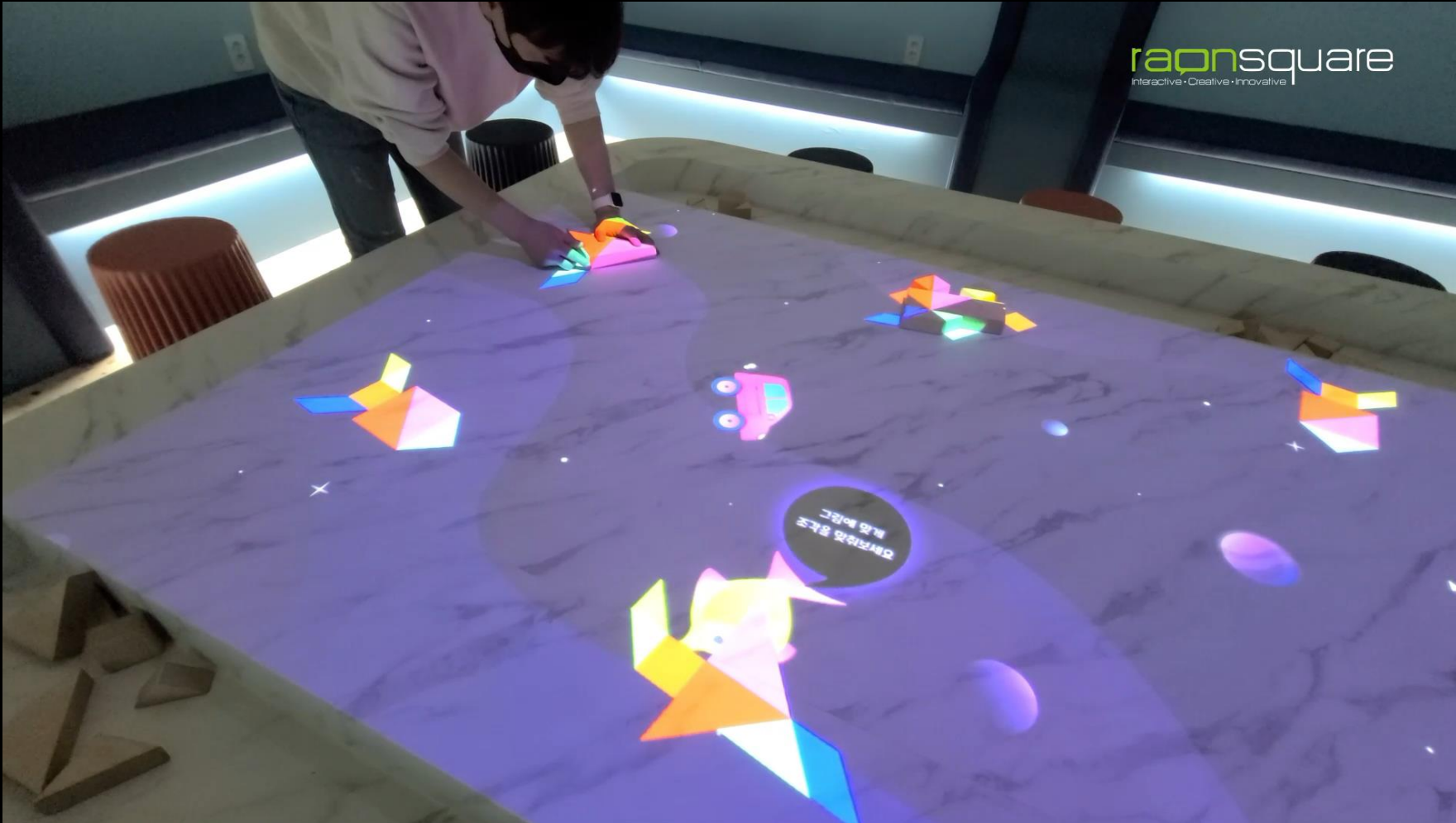
Digital tangram play using a beam projector and an object recognition sensor.
