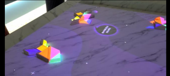
Digital tangram play using a beam projector and an object recognition sensor.
