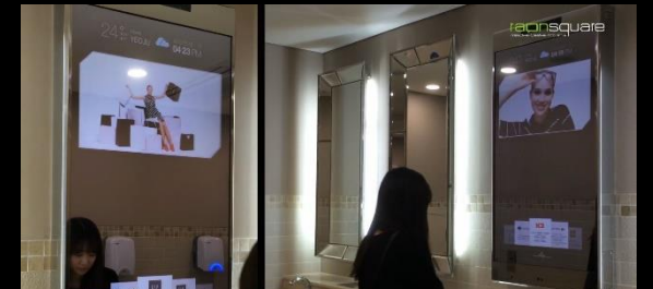
Interactive smart mirrors that leverage proximity sensors to provide contextual shopping information
