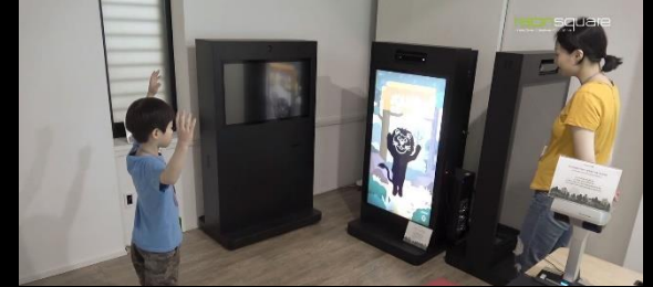
Using motion recognition and joint recognition sensors to create animal shadows. (tigers, monkeys, rabbits)
