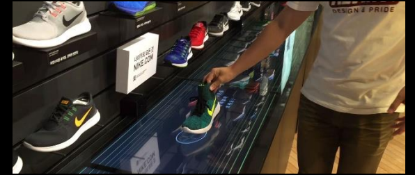
When you lift or release a product, the proximity sensor automatically recognizes the situation and provides information about the product.
